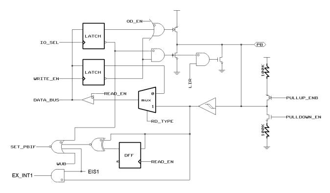
Figure 11 Block Diagram of PB1
