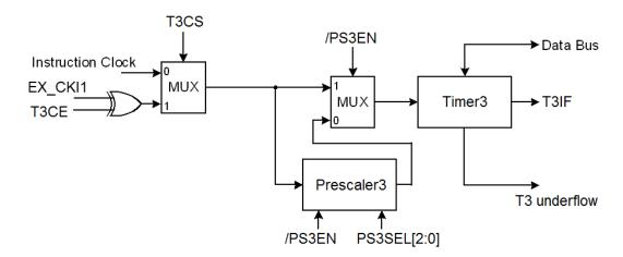
Figure 21 Block Diagram of Timer3
