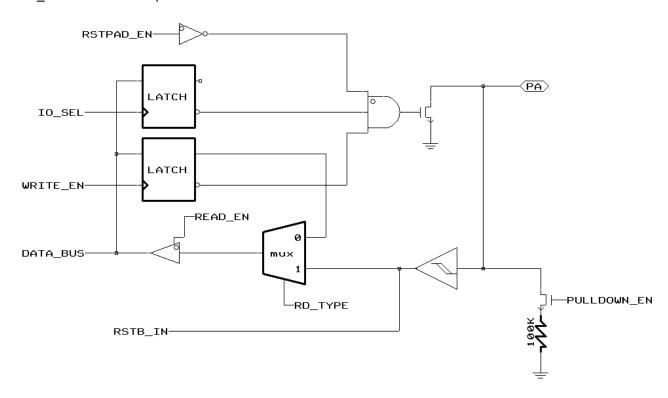
Figure 8 Block Diagram of PA5
