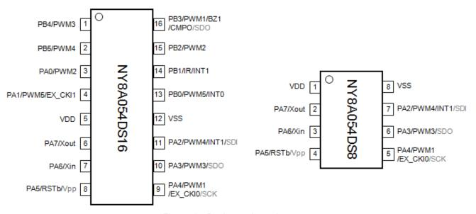
Figure 1 Package pin assignment
