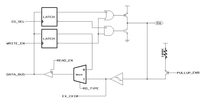
Figure 7 Block Diagram of PA4
