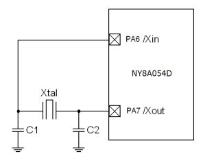
Figure 32 Connection for External Crystal Oscillation
