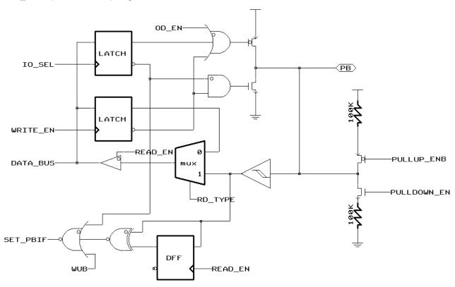
Figure 13 Block Diagram of PB3
