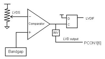
Figure 28 LVD block diagram
