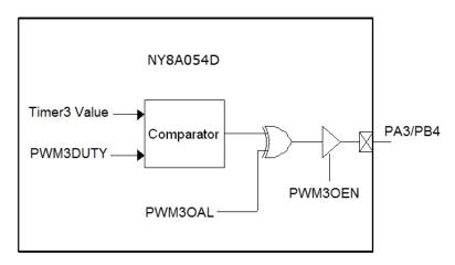
Figure 23 PWM3 Block Diagram
