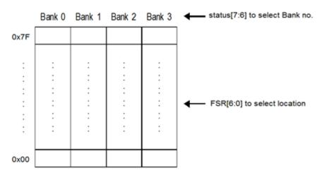
Figure 3 Indirect Addressing Mode of Data Memory Access
