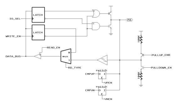
Figure 5 Block Diagram of PA[3:2]&PA0
