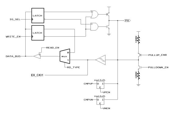
Figure 6 Block Diagram of PA1
