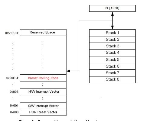
Figure 2 Program Memory Address Mapping
