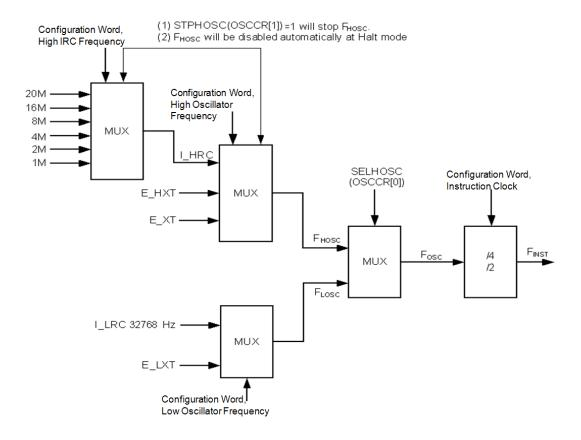
Figure 31 Oscillation Configuration of NY8A054D
