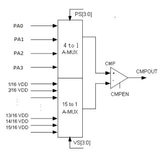
Figure 29 Comparator P2V mode block diagram
