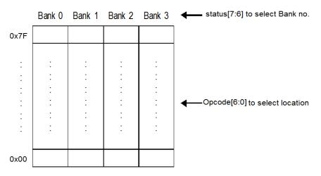
Figure 4 Direct Addressing Mode of Data Memory Access
