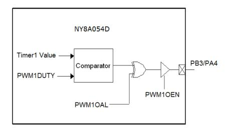
Figure 18 PWM1 Block Diagram
