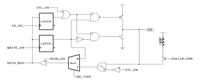
Figure 9 Block Diagram of PA6, PA7
