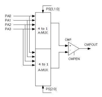
Figure 30 Comparator P2P mode block diagram
