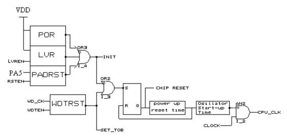
Figure 34 Block diagram of on-chip reset circuit
