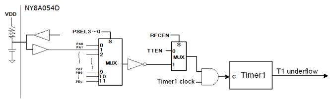
Figure 26 RFC Block Diagram
