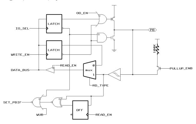
Figure 14 Block Diagram of PB4, PB5
