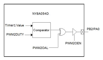
Figure 20 PWM2 Block Diagram
