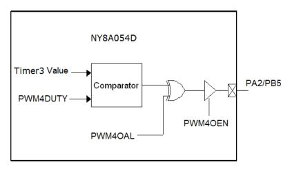
Figure 24 PWM4 Block Diagram
