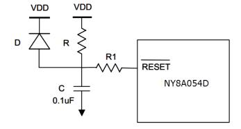
Figure 35 Block Diagram of Reset Application
