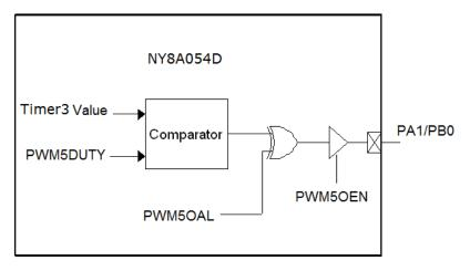
Figure 25 PWM5 Block Diagram
