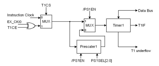
Figure 16 Block Diagram of Timer1
